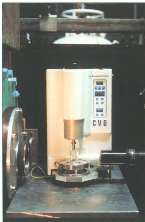
Figure 1: Picture of the BOHLIN Rheometer installed on the small-angle neutron scattering instrument D11.
