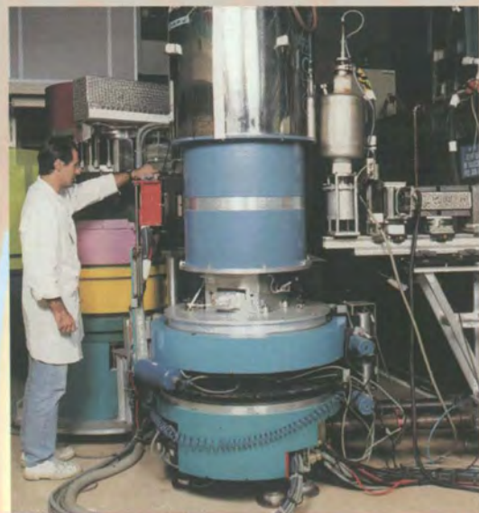
Jacques Previtali, CEA Grenoble, installs the new 4 Tesla horizontal field cryomagnet on IN12.
