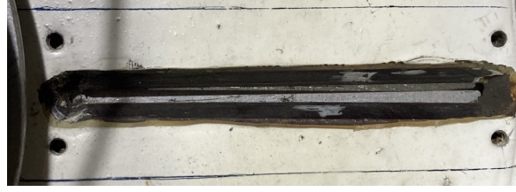
Figure F.6.: One of the open slits of the chopper used for experiment 3-14-323. The slit defining the opening time for neutron is constituted by the black boron rubber and has a width of 3.073 mm. The slit defining the shape of the \gamma -signal is the stadium shaped slit of Gd paint in white.
