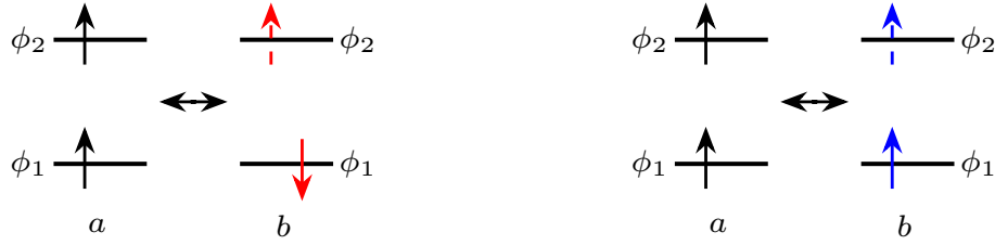
Fig. 1.3. Schematic of the simplest spin-polarised delocalisation (double exchange) mechanism across two sites with S_0 = 1/2 . The spins in \phi_1/\phi_2 prefer to align due to on-site exchange interactions. Thus, there is a energy cost associated with antiferromagnetic coupling between the core spin on sites a/b since the delocalised electron keeps its projection during transfer.
