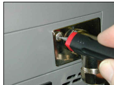
Remove plate holding the armoured cable connection (8)
