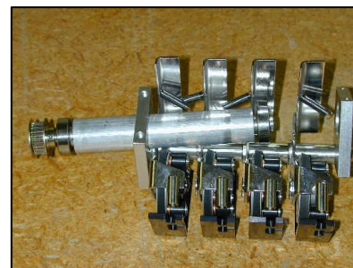
Main roller removed - bar holding pump head supports can be seen
