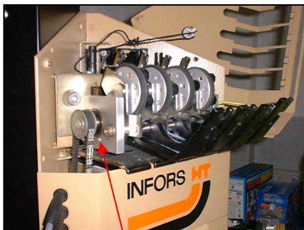
Side view showing drive belt -10
