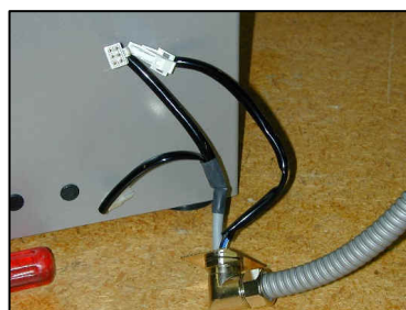
Motor cables removed from base unit (9)
