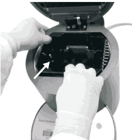
Fig. 2: The reaction chamber can easily be removed from the incubator unit for cleaning. The temperature sensor (indicated with an arrow) fits into the hole at the bottom of the chamber in one orientation only.
