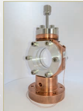
Transparent sample cell for UCN transmission experiments developed as part of my PhD work.
