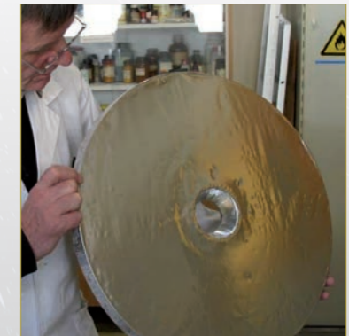
Top - Graph of neutron reflectivity from reflectors of different types. Bottom - Example of a reflector with a nanostructured surface.
