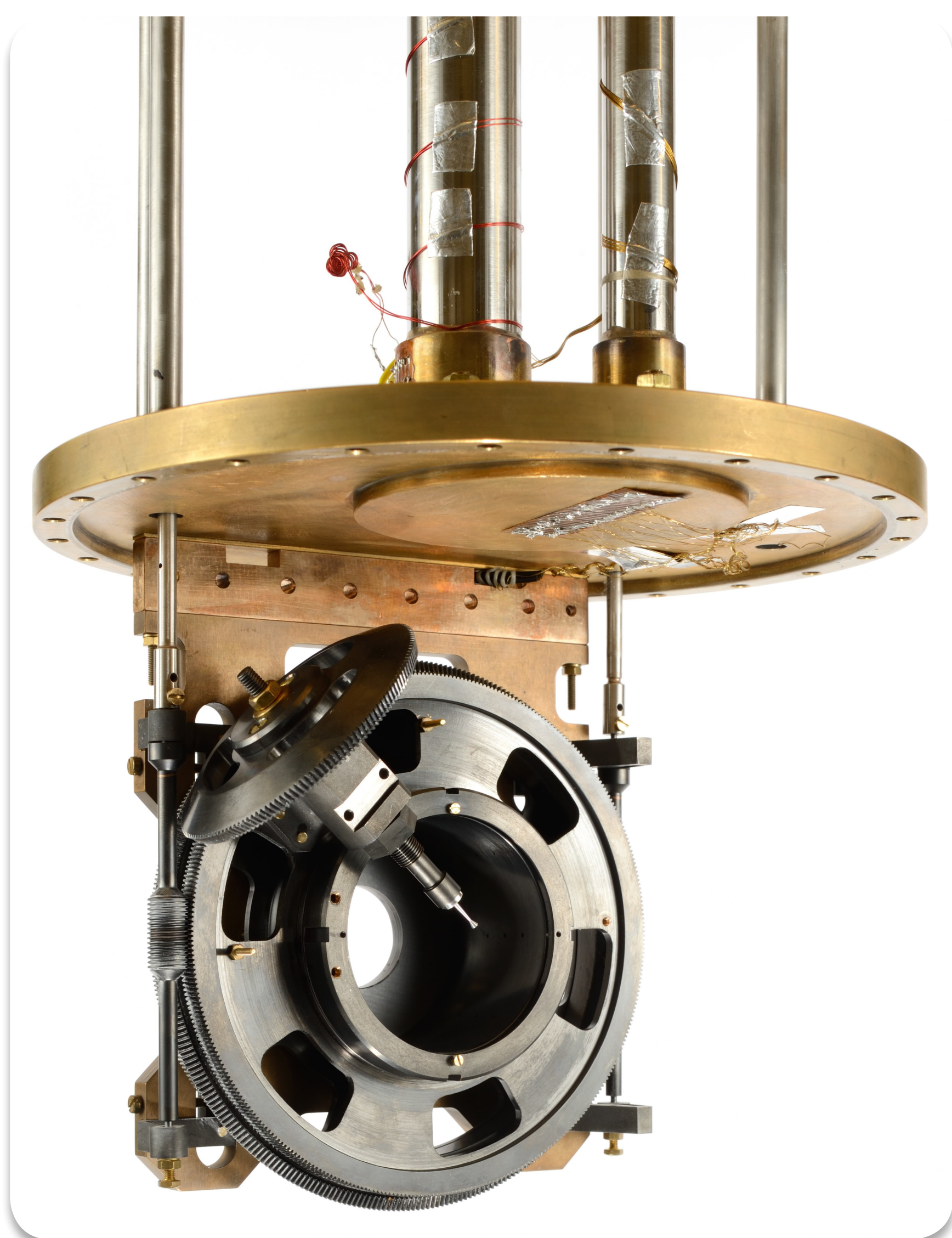
The non-magnetic Eulerian cradle mounted inside the 3 K pulse-tube cryostat. © Ecliptique – Laurent Thion
