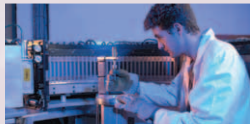
High-resolution powder diffraction is used to analyse polycrystalline materials
