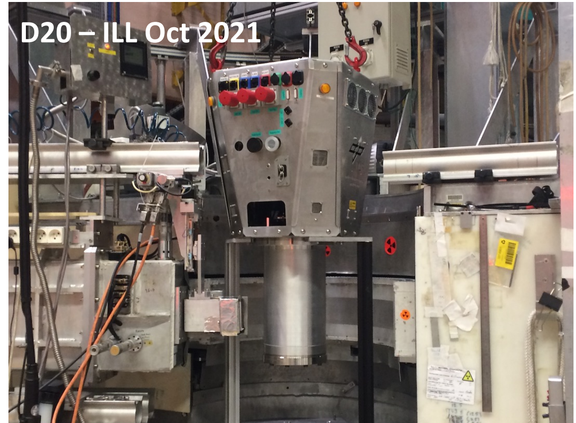
Spin-off from MAPHEUS: Compact plug+play levitator (Synchrotron/Neutron Sources)
