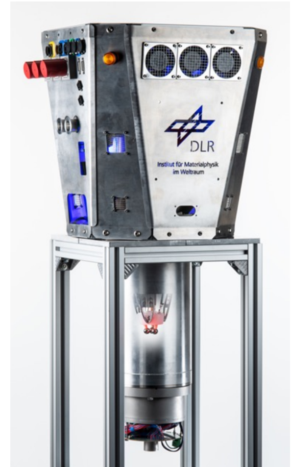
compact, robust, plug&play ESL for neutron/X-ray scattering
