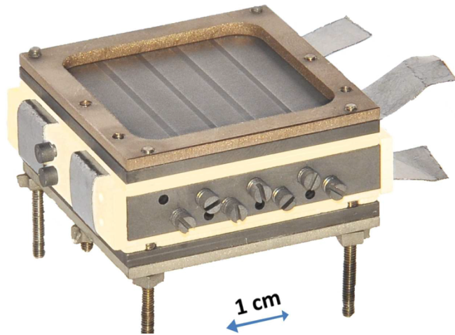
compact and X-ray transparent 1500°C shear-cell furnace
