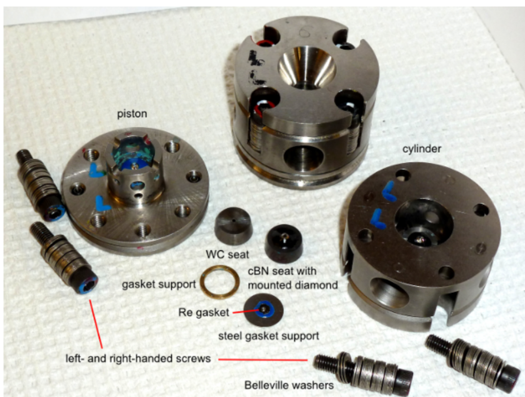
Figure 3.3: Photograph of two symmetric Mao–Bell-type diamond anvil cells belonging to our laboratory at the EPFL. Source: https://epsl.epfl.ch/page-78191.html , accessed on 15.05.2018.
