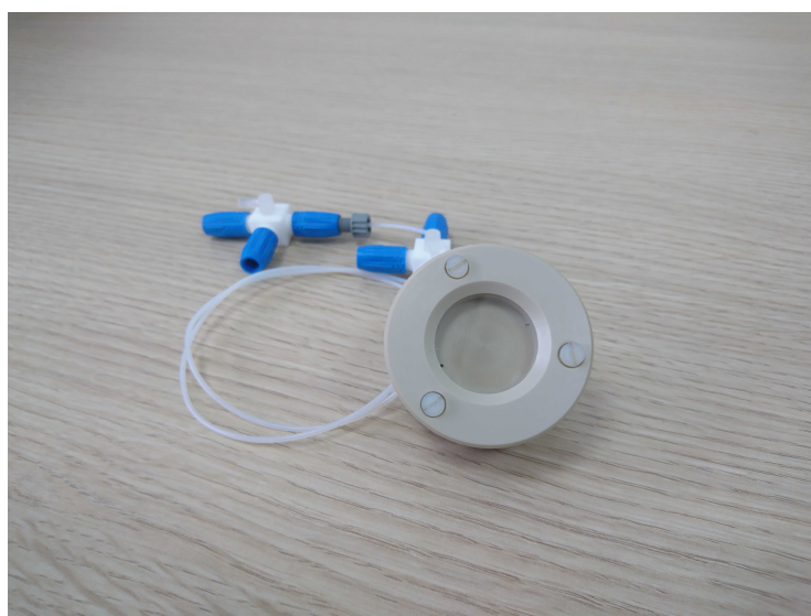
Figure II.2.12 – Solid/liquid cell for fluorescence microscopy experiments.
