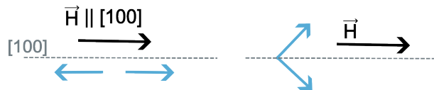
Figure 5.9: Schematic representation of the spin-flop transition observed on the 3-3 super-lattice for field applied along [100] direction. The blue arrows represent the direction of magnetic moments.
