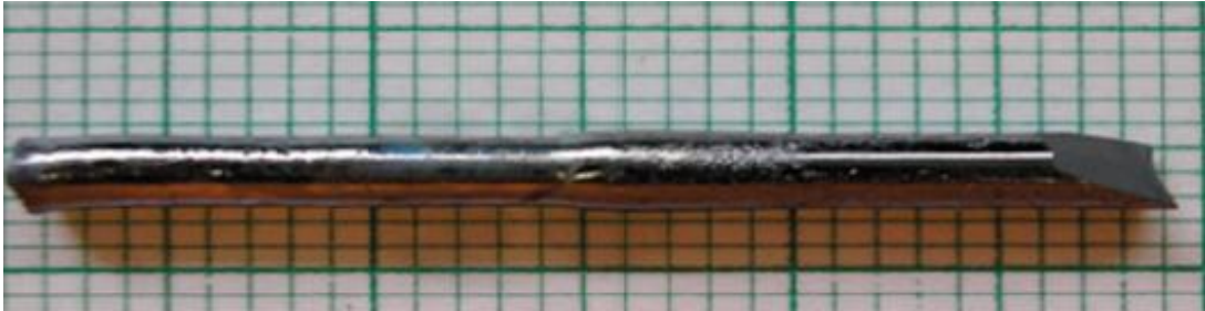
Figure 1.21: Single crystal of \text{BaCo}_2\text{V}_2\text{O}_8 obtained by the floating zone method. The crystals grown by this technique have the typical dimension of about 3 mm diameter and 5 cm long. Figure extracted from [Lej+11].
