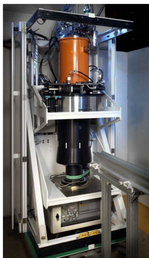
Figure 3.8. Single crystal Laue diffractometer VIVALDI 77 .
