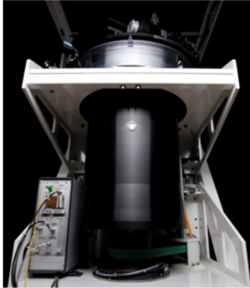
Figure 3.1: LADI-III neutron diffractometer for macromolecular crystallography at the neutron source of the Institut Laue-Langevin (Grenoble) showing the cylindrical detector.
