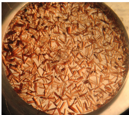
Figure 8.1: Perdeuterated cytochrome c peroxidase crystals employed in the X-ray diffraction work and ultraviolet-visible spectrophotometry experiments. The crystals are in a dialysis button with diameter of 7 mm.
