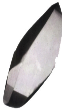
Figure 85. A crystal of saccharide free concanavalin A. The length can be up to 2 mm, and therefore, are suitable for neutron protein crystallography studies, as well as SR protein crystallography.
