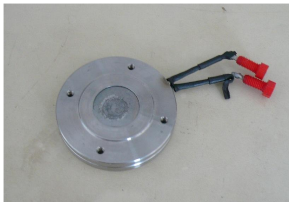
Figure 1.17: Cell for in situ/operando XRPD experiments in reflection diffraction on the PANalytical Empirean diffractometer.
