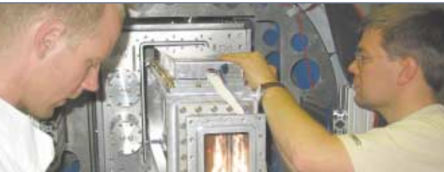
Installing the detector used in the experiment (the TRINE detector)
