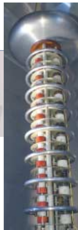
Equipment used to measure the neutron EDM: an array of ultra-cold neutron detectors and the high voltage stack
