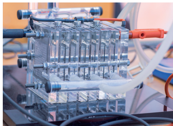
Diagram of a fuel cell based on an anion exchange membrane
