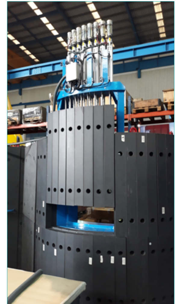
Figure 3 Principal components for PANTHER awaiting installation during the winter shutdown 2018–2019. Monochromator shielding, flight chamber, double-focusing monochromator.
