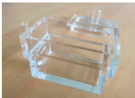
Quartz liquid-liquid cell developed at the ILL and used for neutron reflectivity experiments. The cell is filled in the bottom with water and on top (above the internal quartz edge) with dodecane. The neutron beam passes through 3.5 cm of water.
