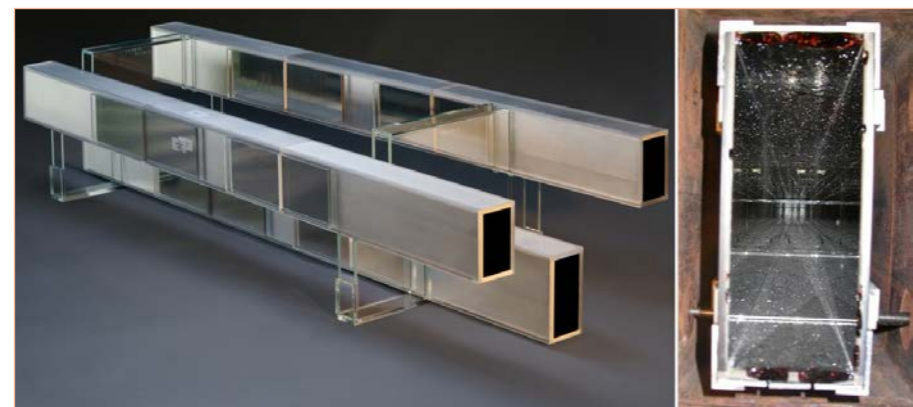
Figure 1 Glass neutron guides: (left) H5: a brand new triple guide; (right) inside of H113, mirror peeling off due to the splintering of the glass below (credits S-DH, SMAE).
