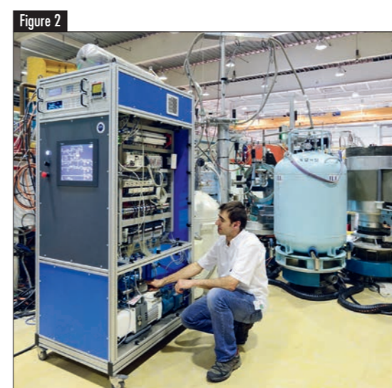
Photo of the complex automated gas-handling system of the closed-cycle dilution system on D10.
