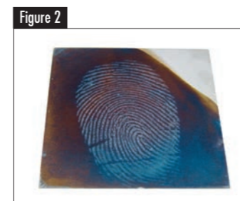
Photograph of a polymer-enhanced fingerprint on a stainless steel surface that was left immersed in water for 7 days before the enhancement treatment, involving electrochemical deposition of polypyrrole.
