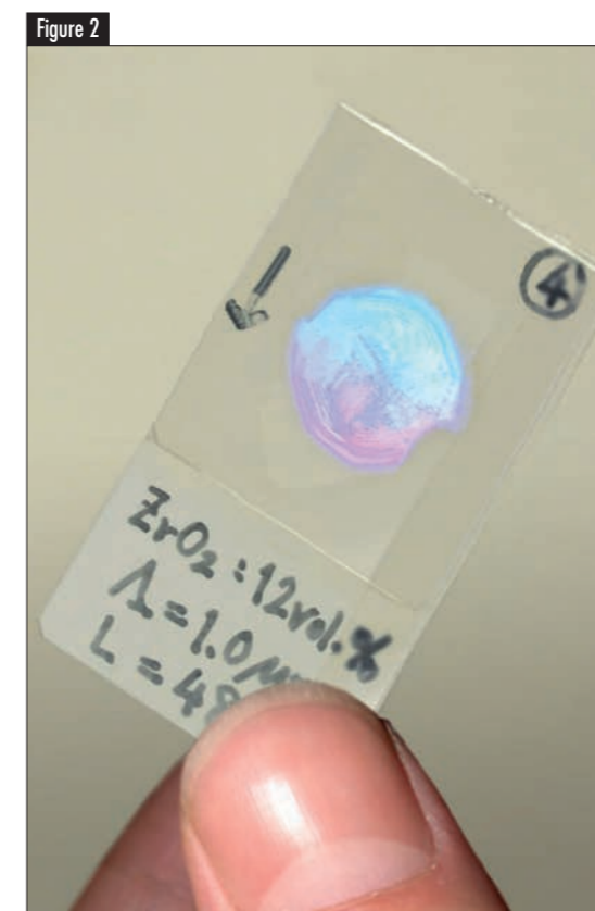
Figure 2 Holographic \text{ZrO}_2 nanoparticle-polymer composite grating diffracting light from a lamp. The grating periods and thickness typically range from 300 to 1000 nm and from 50 to 150 \mu\text{m} , respectively. The sample diameter ranges from 1 to 3 cm. The long-term mechanical stability of the holograms over several years has been confirmed by regularly checking the properties of samples with light.
