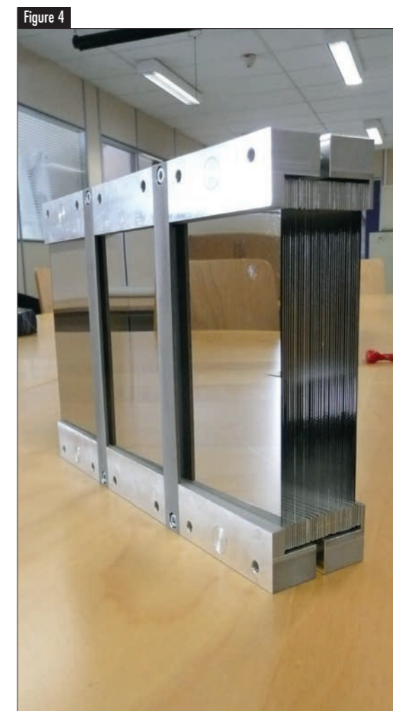
An individual analyser cassette contains 37 mirrors and covers an angle of 1^\circ .
