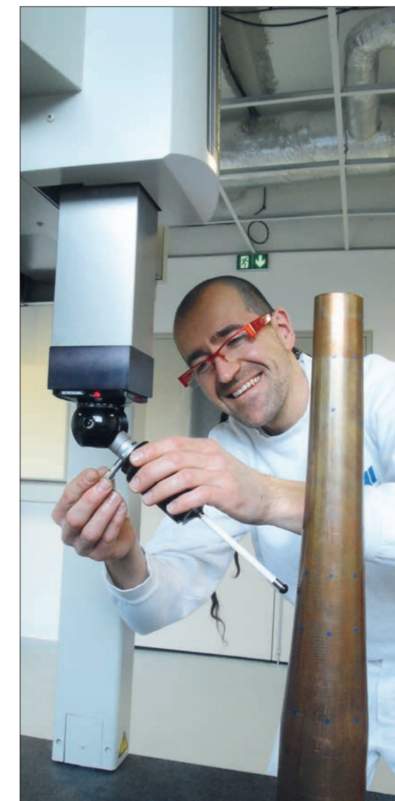
Sergio Garcia Martinez, the technician of the Materials Science Support laboratory, changing the touch probe of the dimensional coordinate measuring machine.
