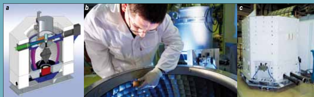
Figure 1: Cross-section view of the LAGRANGE set-up (a), positioning of graphite crystals on the analyser frame (b), and completed spectrometer (c) ready for first neutron tests.
