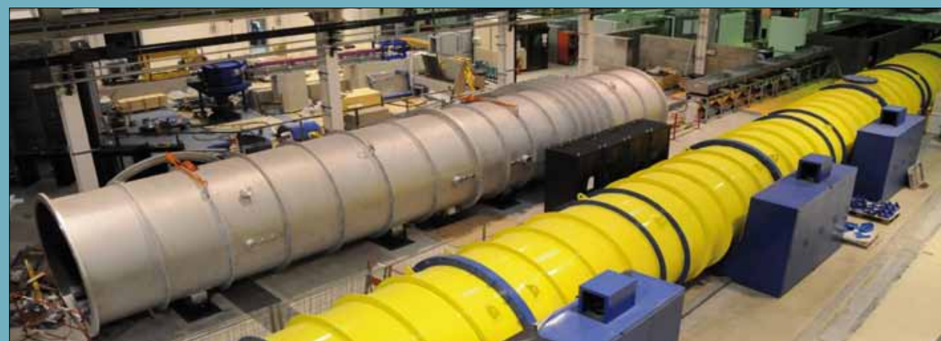
Figure 1: The D33's detector tank (left), lying next to D11 in the newly extended ILL7 guide hall.
