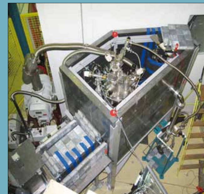
Figure 2: Set-up of the UCN source "SUN-1" at H172A. The cryostat containing the helium converter is situated inside a lead castle. Shown is the set-up with sideward UCN extraction as used in the experiments reported in [4]. The clean room in the background houses the gravitational spectrometer GRANIT under construction.
