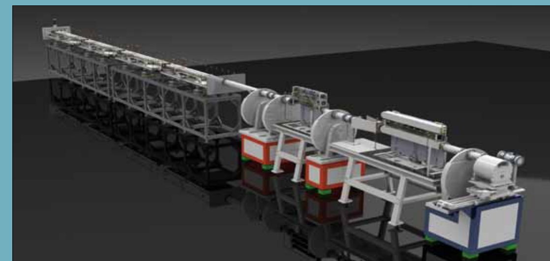
Figure 2: Solidworks impression of the D33 casemate components and collimation housing showing optical components such as the velocity selector, choppers, polarisation components and wavelength filters.
