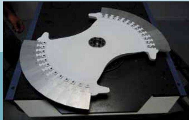
Figure 1: Phase Space Transformation (PST) disc with dummy cassettes on the test drive.
