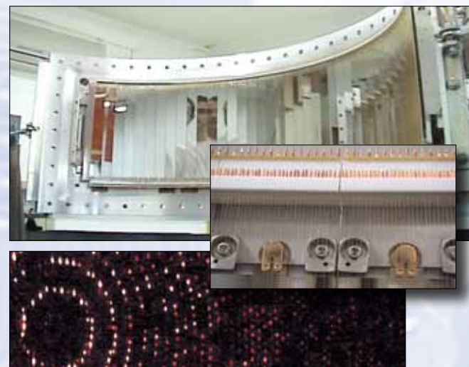
The new D19 detector (top), built by the ILL detector group, subtends an angular range of 120 x 30 degrees, and is the centrepiece of the refurbished instrument. Also shown is a diffraction pattern from a protein recorded using this detector.
