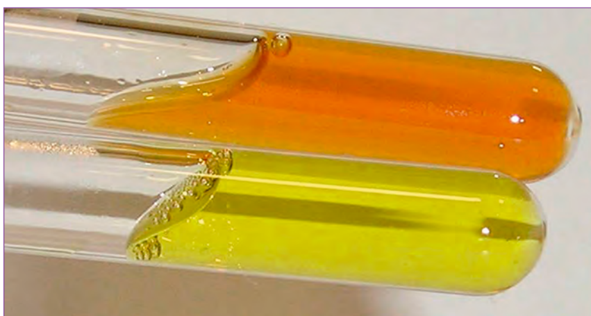
Figure 1: Physical appearance of 10 wt% gelatin plus 0.03M C6PAS samples at 41°C before (lower sample) and after irradiation (top).
