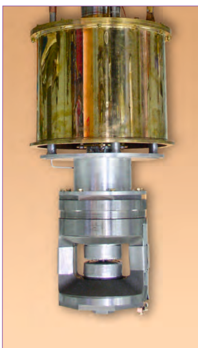
Figure 2: Picture of the ILL Paris-Edinburgh press attached to its dedicated CCR. The systems allow measurements up to 10 GPa in the temperature range 3.5-300 K.
