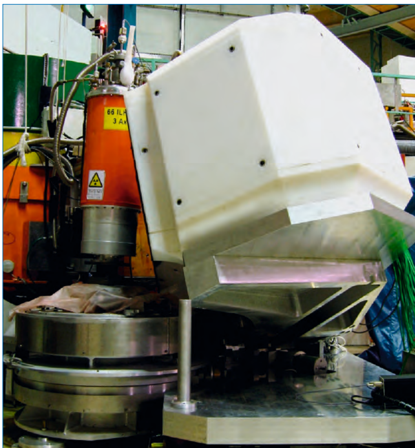
Figure 4: The multiplexed secondary spectrometer FlatCone operating on IN20 .
