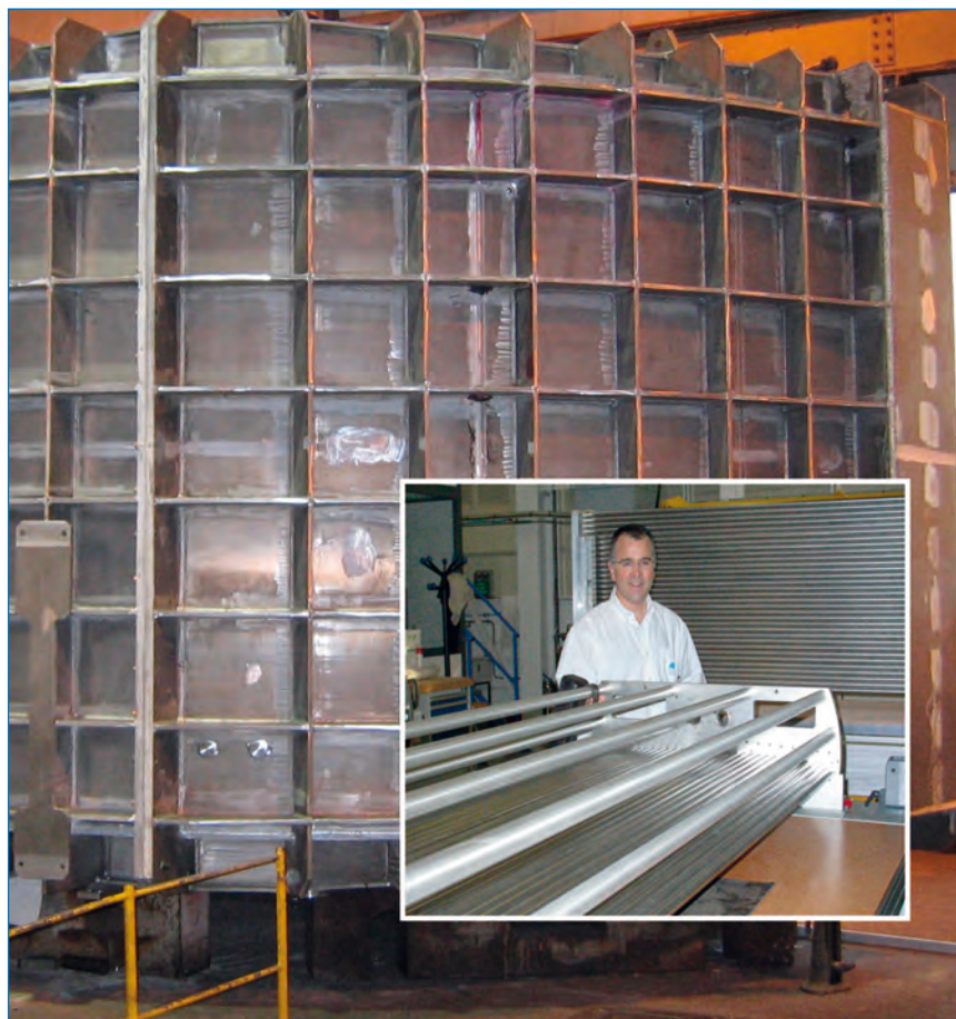
Figure 6: IN5 secondary spectrometer flight chamber with the inset showing one of the cassettes of the 3m position-sensitive detectors.
