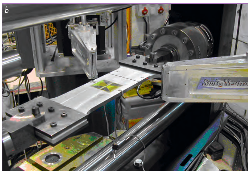
Figure 1: Experimental setup at SALSA for measurement of the stress in a welded plate under fatigue crack growth, measuring a ) in the transverse direction and b ) in the longitudinal direction.
