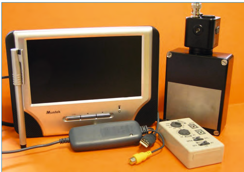
Figure 1: The compact version of the CCD neutron alignment camera with a nominal sensitive area of 80x60 mm, together with its optional 7" (18cm) TFT monitor, alternative USB-2 PC adapter, and electronic exposure controller.
