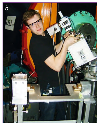
Figure 2: (a) The high-pressure SANS sample holder (volume: 10 cm 3 , temperature range: 0 - 80°C, pressure range: 1 - 300 bar). (b) The cell is dismantled from the neutron beam of D11 for preparing a new sample. The pivot-mounted holder for the high-pressure cell is shown in the foreground.
