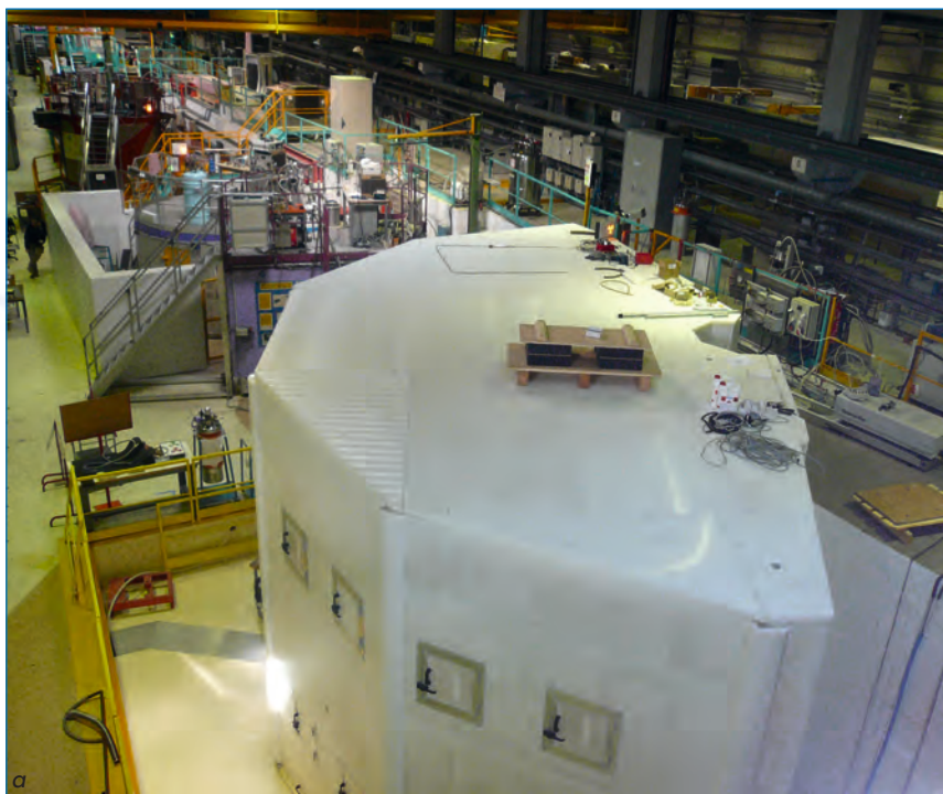
Figure 3: IN5 with its new neutron shielding as seen from above (a). The inside of the protection shows the aluminium frame and the neutron absorber (b). The windows will allow direct access to the detector electronics mounted on the back of the flight chamber.
